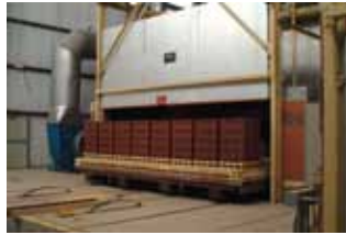
Figure 4. Brick exiting tunnel kiln
