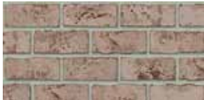
Figure 8. Sand-struck, hand-molded Type FBA brick
