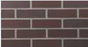
Figure 7. Extruded brick, Type FBX, with a die skin
