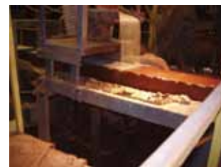
Figure 3. Application of coating to extruded brick
