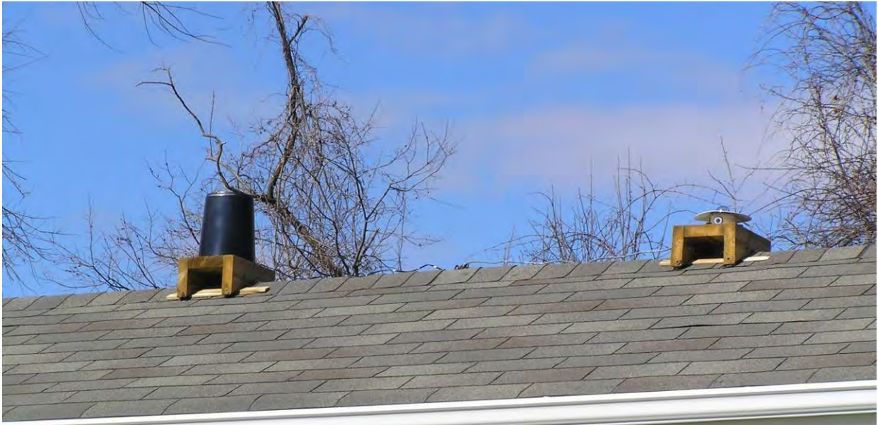
Rain gauge and horizontal solar radiation sensor
