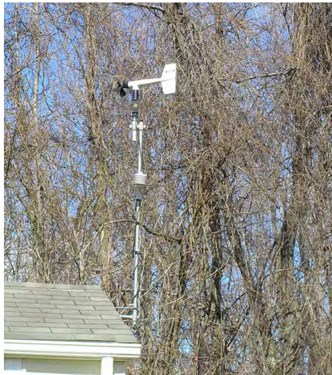
Anemometer, temperature humidity sensor
