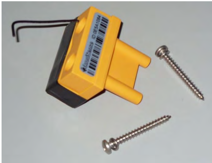
Figure 2. Wireless temperature, humidity, and wood moisture sensor
