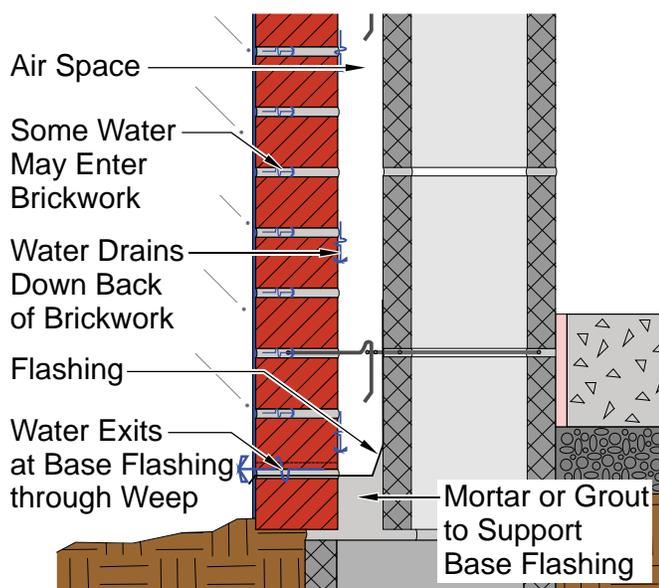
**Figure 1: Drainage Wall Systems.** BIA recommends the use of drainage wall systems, as shown above. BIA does *not* recommend the barrier strategy of filling a collar joint between masonry wythes because it places a source of salts in direct contact with the brickwork.
