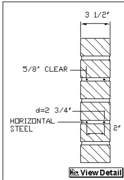
Section Through Four Inch Brick Wall
