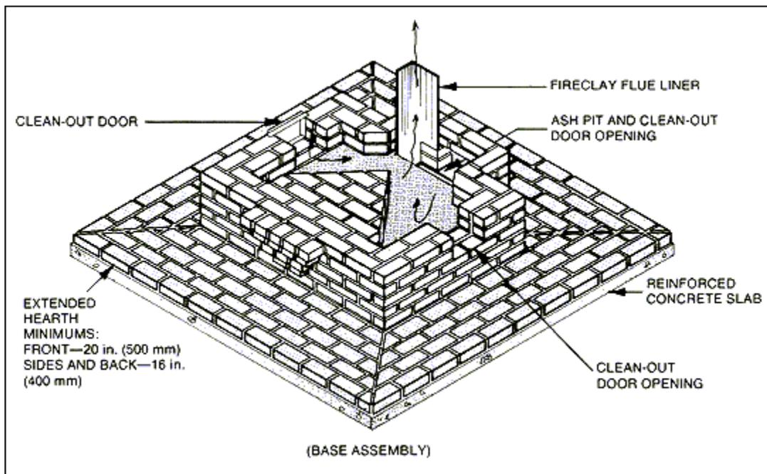
**Fountain-Style Brick Masonry Heater, Isometric**
