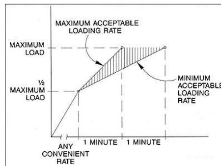
**Compressive Test Loading Rate**
