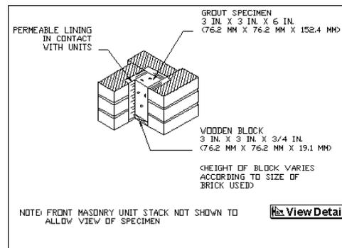
**Grout Mold Using 2 ¼ in. (152.4 mm)
