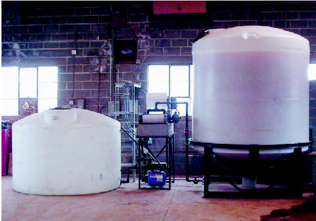
Glen-Gery Mid-Atlantic Plant's brick saw water recycling system consists of a wastewater storage tank, paper filtration system and treated water storage tank.
