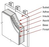
Substrate (e.g., plywood) Adhesive/Attachment Insulation Board
