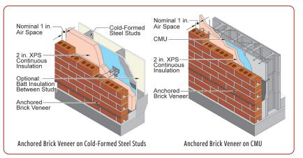
radiant barrier or a reflective coating with an emissivity of 0.05 adjacent to a nominal 1-inch airspace can provide performance equivalent to adding continuous insulation with an R-value of 2.6 to a wall. And the best-performing system of all is brick veneer with continuous insulation over concrete masonry, exceeding the performance of brick veneer over cold-formed steel studs by 24% to 41%, depending on the presence of batt insulation in the stud cavity.
