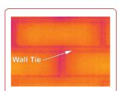
Veneer ties are not visible in infrared (IR) photos taken during hotbox testing, illustrating that ties are not thermal bridges.
