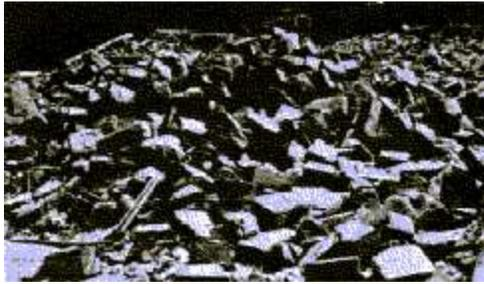
**When existing walls are demolished, hard-burned brick and salmons are hopelessly mixed. It is virtually impossible to distinguish between durable and non-durable units.**
