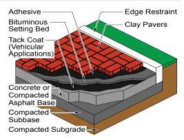
Figure 1 Typical Brick Pavement on Bituminous Setting Bed
