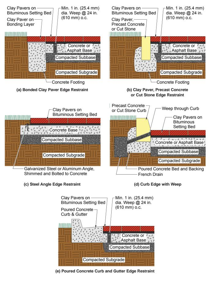
Figure 4 Edge Details for Brick Pavements
