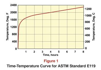
until a failure occurs (termination point is reached) or a designated extent of time passes. ASTM E119 requires that the air temperature at a distance of 6 in. (152 mm) from the exposed (fire) side of the specimen conform to the standard time-temperature curve, as shown in Figure 1.
