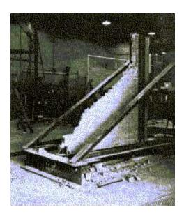
Typical Mode of Failure in Racking
