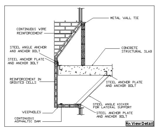
Prefabricated Brick Sill, Spandrel and Soffit
