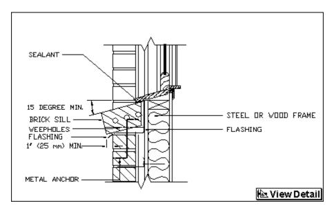
Sill in Frame/Brick Veneer Construction
