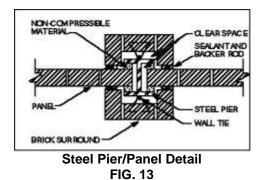
When reinforced concrete or masonry piers are used, the flanges should be analyzed to ensure that the shear and bending forces imposed on them by the adjacent panel do not exceed allowable stresses. If for aesthetic reasons, an exposed steel pier is not desirable, brick can be built around the steel in the form of a pilaster (Figs. 13 through 15). Corrosion protection of the pier should be considered when steel piers are used.
