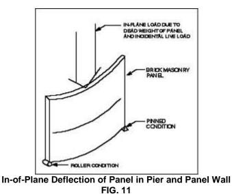
The piers, on the other hand, act as vertical cantilevers and must be designed to resist all lateral loads transferred from the panels. The piers are usually anchored to or embedded in reinforced concrete piles, which vary in depth due to local soil conditions. The piles must be designed to resist all shear and axial loads and the overturning moment caused by the panel due to out-of-plane wind
