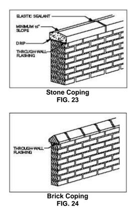
Through-wall flashing is required directly under the coping. The flashing should extend beyond the faces of the wall to form a drip. All penetrations through the flashing made by the anchors must be adequately sealed with a compatible material.
