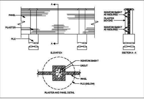
Pilaster and Panel Assembly FIG. 16
