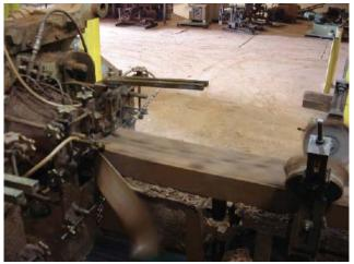
Photo 3 After Mining, Clay is Extruded Through a Die and Trimmed to Specified Dimension Before Firing
