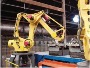
Photo 5 Robotic Arm Unloading Brick After Firing
