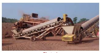
Photo 1 Clay or Shale Being Crushed and Transported to Storage Area
