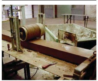
Photo 6 Some Brick Textures are Applied by Passing Under a Roller After Extrusion
