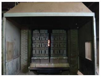
Photo 4 Brick Enter Tunnel Kiln for Firing
